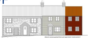
Front Elevation - North (1:100) Allow to remove painted finish and repair bricks / mortar joints if visible when viewed from this angle
